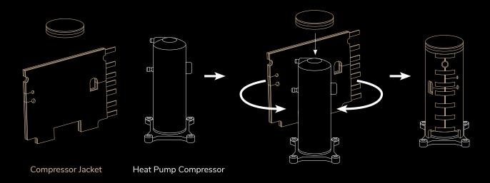
Customized multilayer sandwich structure with sound barrier.
