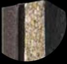
**Meluton Reduce® Pro+ PUR A8** Combining the Basic and the Pro model, the Pro+ provides you with the best noise insulation on the market. Use it on surfaces near the source of the sound whenever you have 65mm of installation space. Attach the materials together with the self adhesive surface and strenghten the attachment with Sikaflex.
